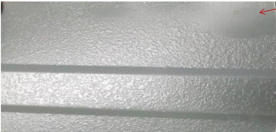
Close up image of severe "Wet Stack Corrosion". Note smooth, normal surface in upper right corner.
